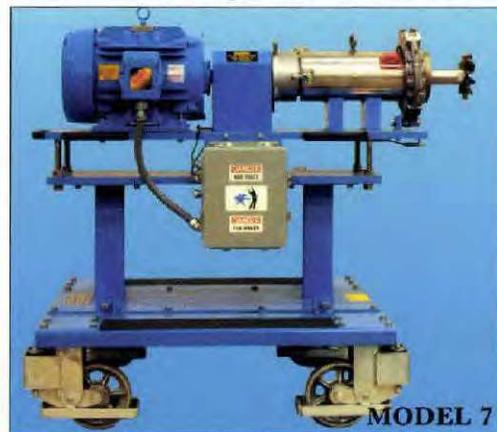
**G**ala's Model 6 and 7 pelletizers employ a manual hand wheel to adjust the blade to the die face. These models are used to produce pellet rates up to 12,000 lbs/hr (6,000 kg/hr) and are capable of cutting a wide range of polymers - from hot melt adhesives and TPR to polyester and nylon.
