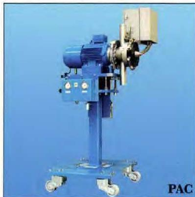
**T**he design of the PAC (Pneumatically Adjustable Cutter) is similar to that of the standard SLC (Spring Loaded Cutter). The PAC has a spring-loaded blade holder connected with a driven shaft in such a way that it can be shifted in an axial direction. The blades are pressed against the die plate at the optimum pressure for the current operating condition. This allows cutting pressure to be increased during start-up, then decreased to the minimum pressure needed during normal operation.
